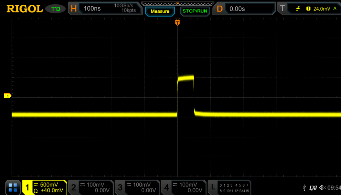
50 ns Narrow Pulse, Full Bandwidth
