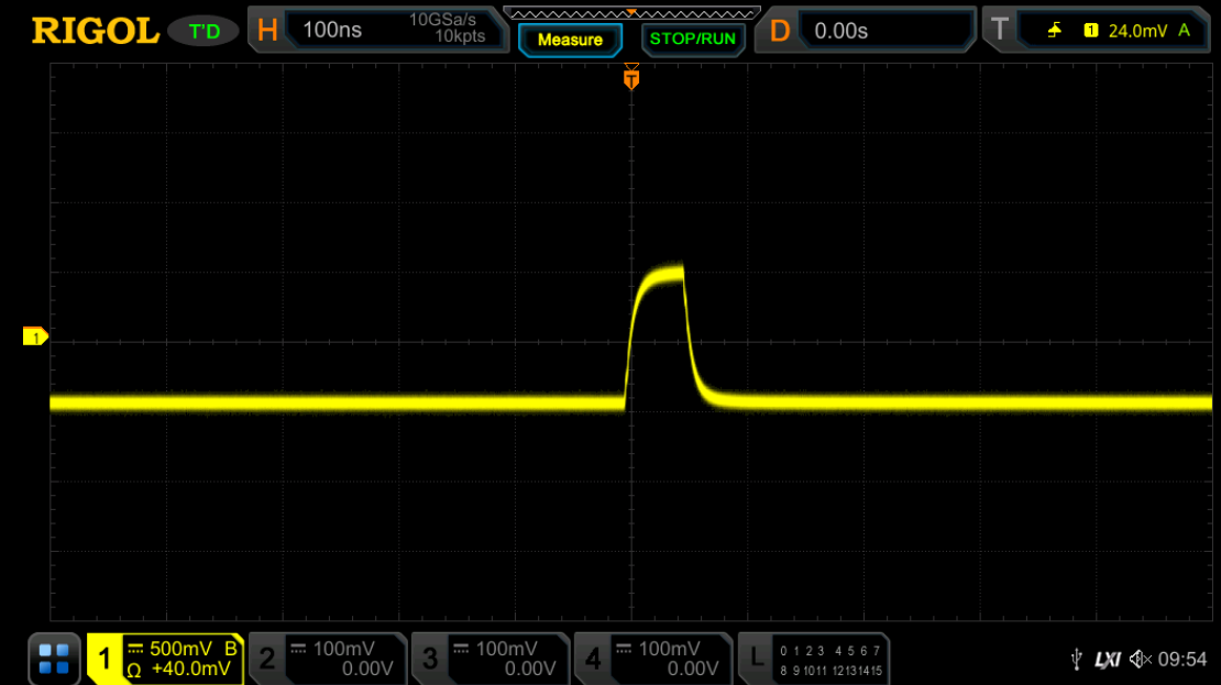
50 ns Narrow Pulse, Insufficient Bandwidth
