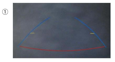
Once putting the gear to reverse, the lines appears in the screen automatically.
