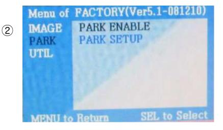
② When pressing ▲ → ▼ → ▲ → MENU buttons in sequence, OSD menu appears like left picture. At this, once selecting "PARK SETUP" with pressing 'OK' button in the remote, you can control distance between 2 parallel lines.
