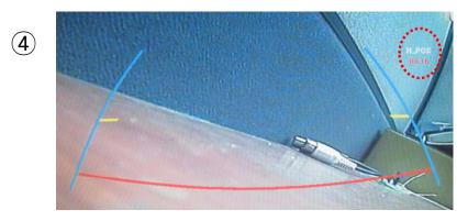
④ After Step. 3, press ▲, ▼ buttons of the remote to control left, right position with pressing 'OK' button, and then you can control up, down position
